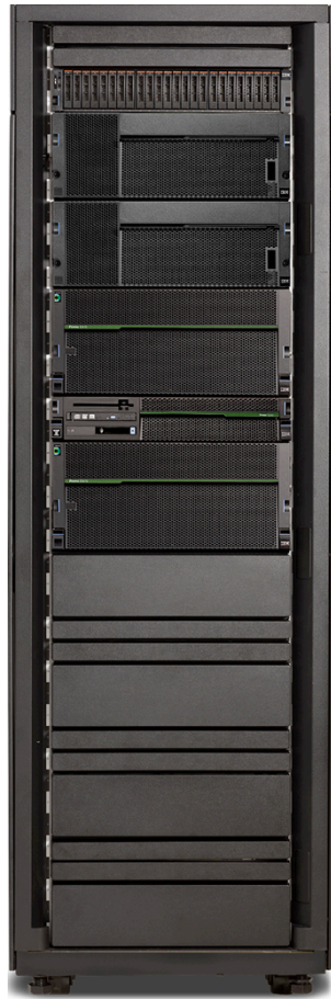
19-inch Rack (E870 Shown)
